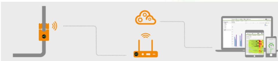
Sensors report the power consumption to the bridge. The bridge, in turn, transfers the circuit level information, along with readings originated by the utility meter and read through a pulse input on the bridge, to the cloud, the solution's cloud-based analytics platform. A single bridge can collect data from up to 250 sensors and two utility meters, and multiple bridges can be used in a single site to increase coverage.
